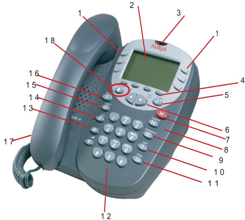
1 - Call appearance feature buttons: Used to access incoming/outgoing lines and programmed features.
