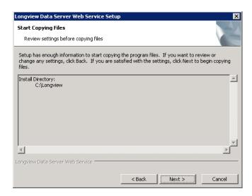
11. Review the settings, and then click Next. The Installing page opens, displaying the progress of the installation process.
