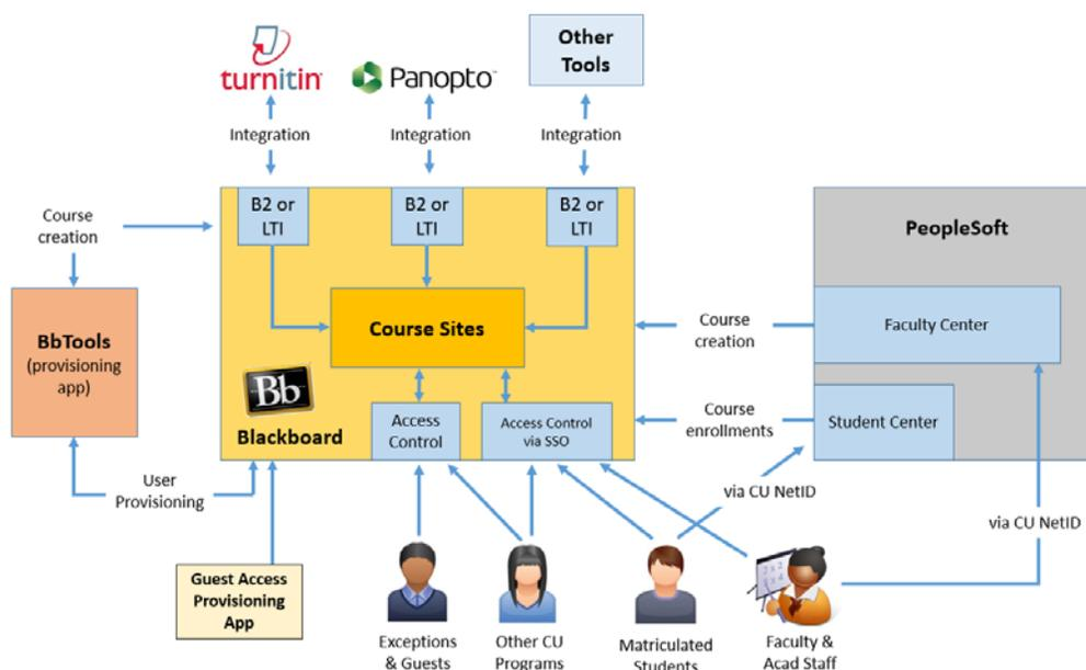
Figure 101. Technical diagram depicting the LMSs connections with other systems
